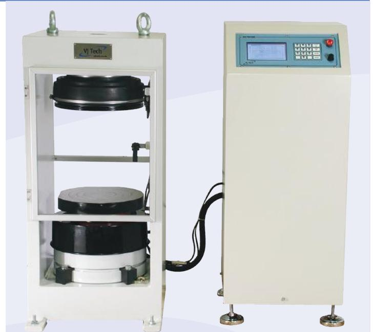
VJT51-2011 - 2000kN Automatic Concrete Machine (Autocon)
